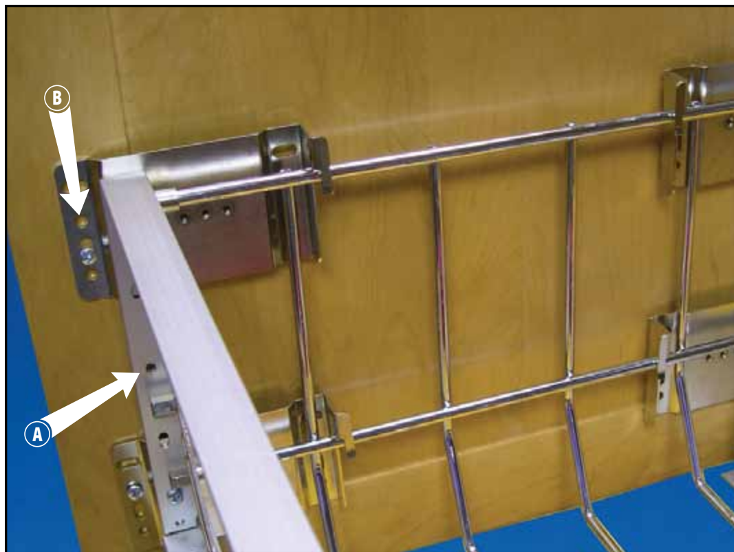
View of circumstances requiring 5345-DM-KIT. Notice how stock mounting position would place wood screws dangerously close to the edge of the door frame (A), which may cause the wood to split. With the Door Mount Extension Brackets you can safely affix the door using a much stronger area (B).
